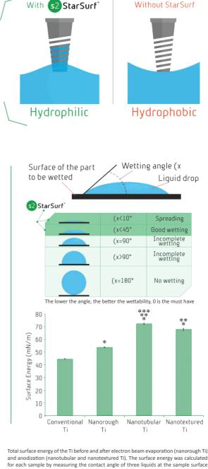
Total surface energy of the Ti before and after electron beam evaporation (nanorough Ti) and anodization (nanotubular and nanotextured Ti). The surface energy was calculated for each sample by measuring the contact angle of three liquids at the sample surface and entering values into the Owens-Wendt equation. Values are mean  $\pm$  SEM; n=4, \*p < 0.01 compared to nanotextured Ti; \*\*p<0.01 compared to nanorough Ti, \*\*\*p < 0.05 compared to nanotextured Ti.
